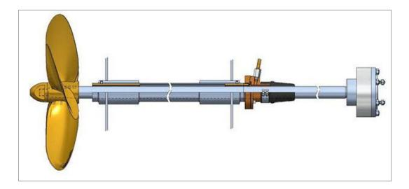
The next component is the intermediate shaft. There is no specific restriction on the number of intermediary shafts that a ship can have. However, beyond 2 shafts, it's difficult to service and maintain. The reason for this is the large catenary force acting on the entire propeller shaft. This force deforms and damages parts because of their weight.
