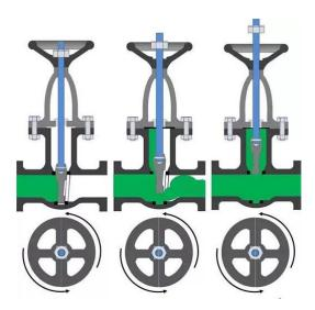
Marine Gate valves material is cast iron, cast steel and cast copper. It is suitable for occasions requiring low flow resistance and low medium pressure, as well as large-diameter pipelines such as seawater, fresh water, fuel oil, and lubricating oil.
